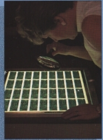
Shirley Smith uses a magnifier to inspect circuit boards.
