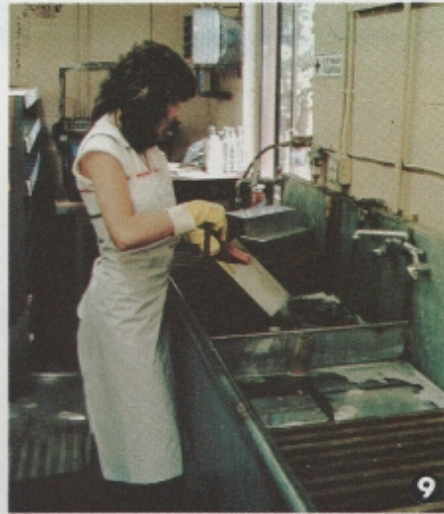
One of our machines is being used to bend the sheet metal into the proper shape. After the sheet metal is bent, it is sent to the paint shop where it is etched in a large tank to make sure that the paint will adhere to the aluminum. It is then sent to the painting area where a very high quality paint is applied. See 9 and 10.
