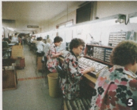
The P.C. Board area is where the printed circuit boards are "stuffed" with the electronic components, especially chosen by White's for their high quality.
