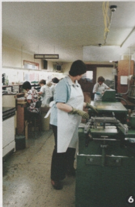
Shown here is the Electronic Automatic Soldering Equipment, "Solder Wave Machine", skimming over the top of a "river" of molten solder. See Photo #7
