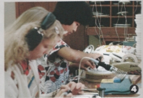
Actual Loop Assembly process. The loops are placed inside the foam holder and then soldered to the loop cable which plugs into the detector housing. This type of loop shown here, is a revolutionary new loop design, pioneered by White's Electronics. The loop is Patent Pending for the fantastic capabilities of eliminating the back reading problem for all practical purposes that is present in almost all other TR type loops. The back reading problem is a bad object which will appear or read as a good object when it gets close to the bottom of the search coil.
