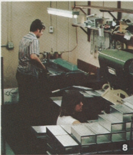
One of our machines is being used to bend the sheet metal into the proper shape. After the sheet metal is bent, it is sent to the paint shop where it is etched in a large tank to make sure that the paint will adhere to the aluminum. It is then sent to the painting area where a very high quality paint is applied. See 9 and 10.
