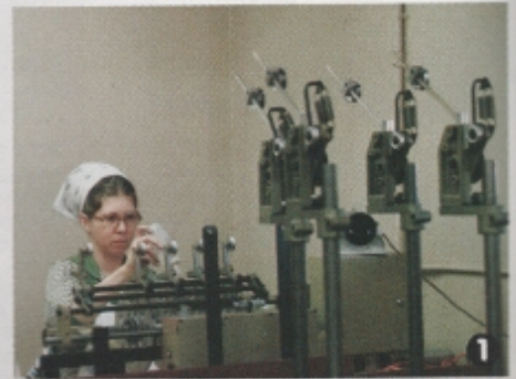
Here you see the operation of taking the bare wire and winding it on four spools simultaneously, which are used as the search coil or sensing device for the electronic metal detector.
