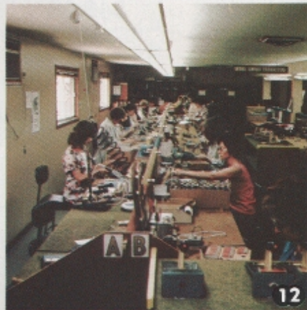
FINAL ASSEMBLY AREA - The Assembly building is where circuit boards are installed into the aluminum housing and loops are then attached, so the unit can be tested to insure that all components are operating properly.
