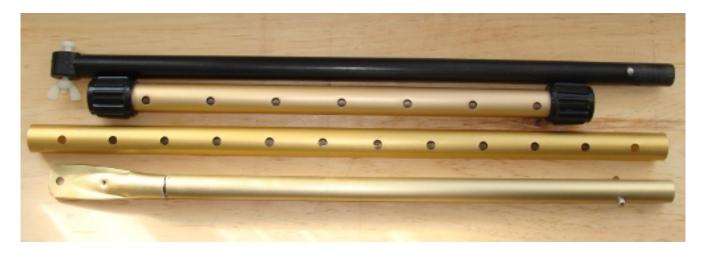
Stem section-- cut off stem coil mount from vintage lower section, will be used as a coupler that will slide into the Fisher middle section and mate with the the vintage middle section that will now become a rear section. Cut to desired length.
