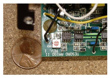
**Step 1**Take your needle nose pliers and gently squeeze the sides of the metal trimpot frame. The frame will lift off. Remove the o-ring.
