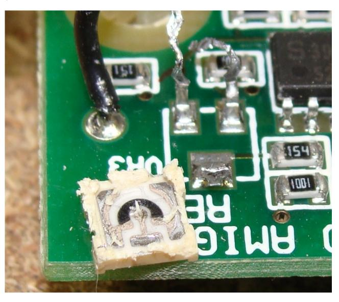
**Step 5**Snip the leads close to the circuit board. Solder a length of 28 guage wire to each pad. You need to do this quick so not to heat up any surrounding parts and damage them.
