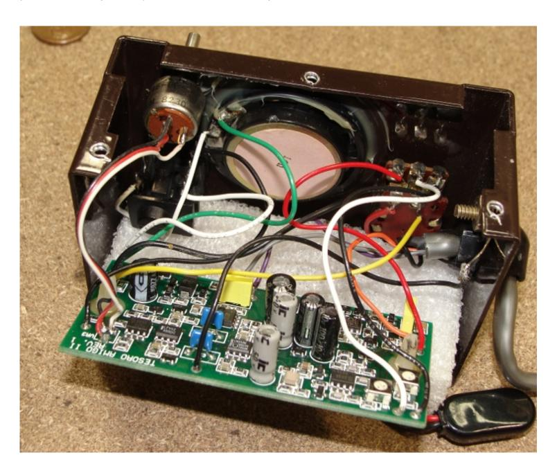
**Step 9**Attach your external pot, and carefully reassemble the box in reverse order. Add a knob to the pot, and off you go.
