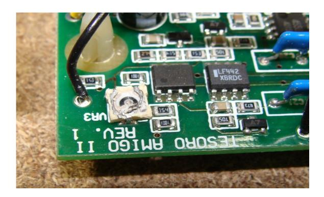
**Step 3**Work the lead traces loose with your forceps and bend each one upward away from the trimpot.
