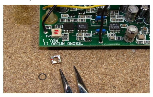
**Step 2** Again, stressing, very carefully breakaway the top of the trimpot, it will reveal 3 metal trace leads.
