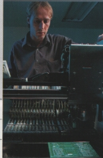
Circuit boards are produced utilising computer driven pick and place machinery to maintain 100% accuracy...
