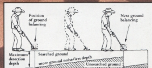
With conventional detectors, ground noises reduce the effective searching depth when you move from where you last ground balanced. Shaded area shows ground not properly balanced.
