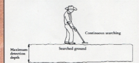
With the automatic ground-tracking feature, you cover the ground faster and more effectively. You don't lose detection sensitivity or depth.
