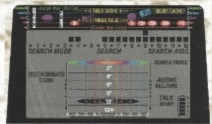
This image shows that an aluminum 12 oz. drink can at 10" has been detected. (9D)
