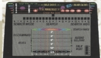
This image shows that a large object, possibly a gold cache has been detected at 12-plus inches. (6.5E)
