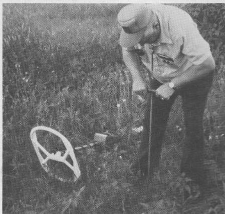
After metal detector gave metal reading indicating possible location of bottle dump, Roy Lagal probes to determine presence of bottles.
