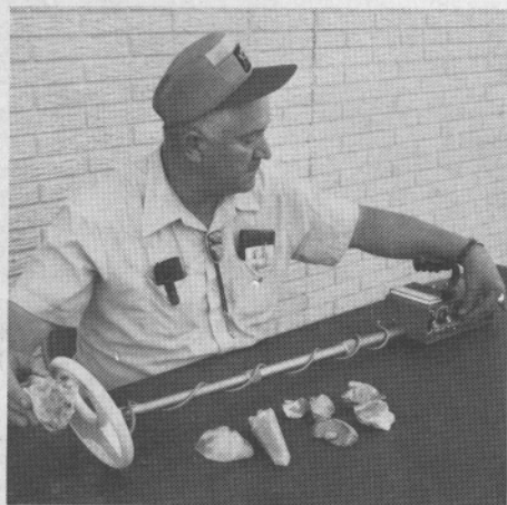
Metal/mineral ore sample bench testing.
