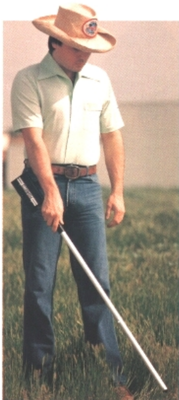
The FX-3 is extremely sensitive to objects with large surface areas, highly magnetized objects and long objects buried vertically.
