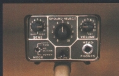
Only three controls and two switches do it all. The dual knob ground reject control has a small single turn coarse adjust knob and a large sixteen turn fine adjust.
